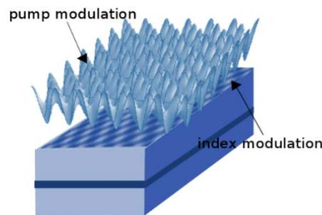
Figure 1. Schematic illustration of a modulated BAS source. The pump (gain/loss) modulation can be achieved by structuring the electrodes and the index modulation by structuring the medium.
