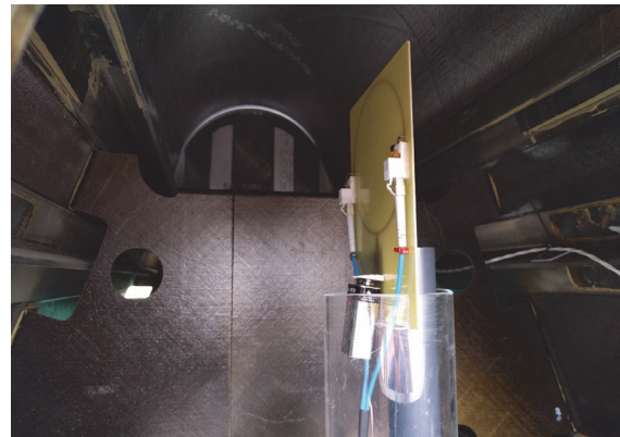
Fig. 8. EH-Field probe measuring the vertical component of the E-Field within the composite fuselage of the INTA Milano
