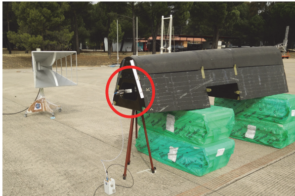
Fig. 6. INTA MILANO test set-up view when the D-dot is placed inside the fuselage
