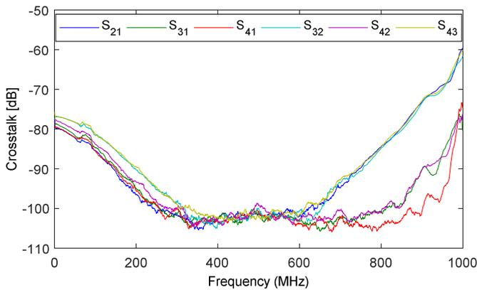
Fig. 7. Crosstalk evaluation of a Full TDEMI measurement system.
