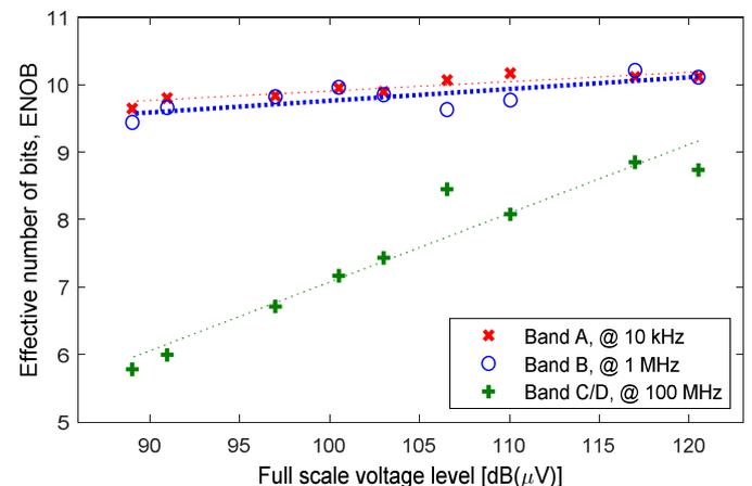
Fig. 5. An effective number of bits of a Full-TDEMI measurement system.
