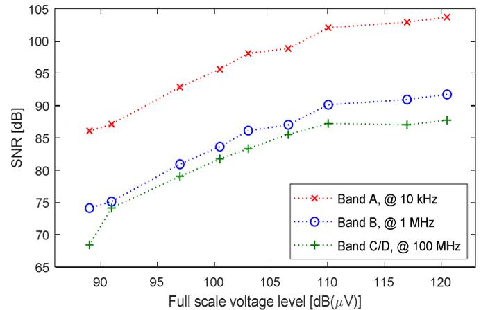
Fig. 4. Signal to noise ratio of a Full-TDEMI measurement system.
