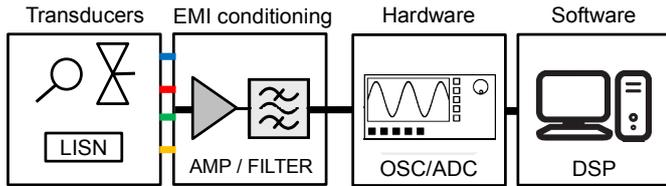
Fig. 1. Block diagram of a Full Time-Domain EMI measurement system.
