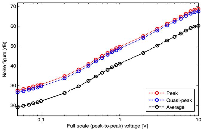
Fig. 2. Noise figure referenced to a RBW of 1 Hz for a Full-TDEMI measurement system based on the oscilloscope Tek DPO5104B configured for having 1 GHz of bandwidth and a sampling rate of 5 GS/s.
