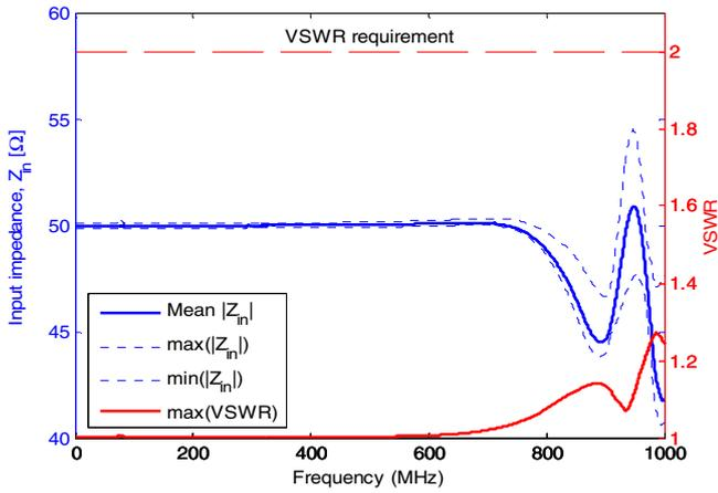
Fig. 6.  $Z_{in}$  and VSWR evaluation of a Full-TDEMI measurement system.
