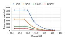
Fig. 1. Effective TR as a function of the worst-case inter-core XT in 22-core MCF.
