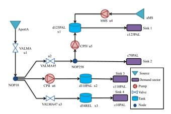
Fig. 1. Drinking water network diagram (Three-tanks).
