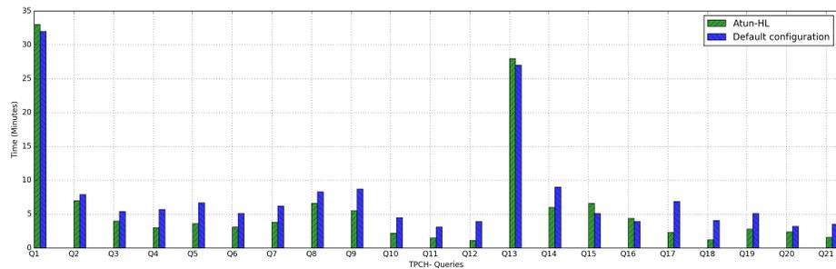
Fig. 7: Improvement in query execution time for 64GB scale factor
