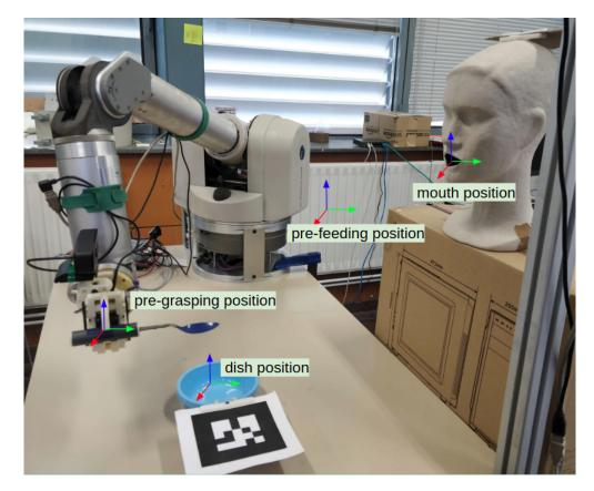
Figure 6.4: Relevant reference positions during the feeding process Source: Own compilation
