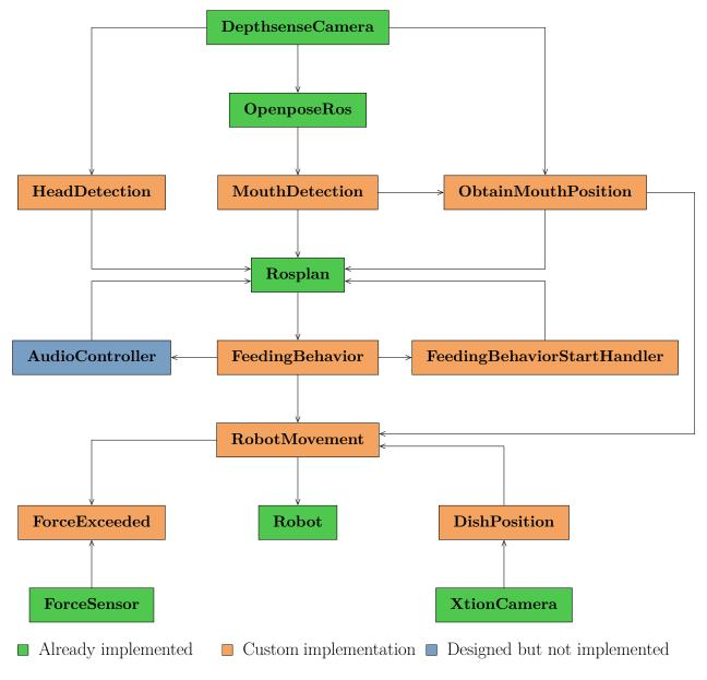
Figure 6.1: ROS Architecture of the feeding assistance implementation Source: Own compilation
