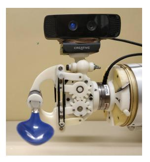
Figure 4.2: 3D printed gripper with camera and force sensor attached Source: Own compilation
