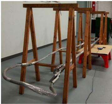
Fig. 5. a) The tested bolted mechanical connector with the entire setup, including bus bars, sensors (1: Hall effect sensor, 2-3: voltage drop terminals, 4: DAQ) to measure and data acquisition modules. b) The loop used to test the power connector.
