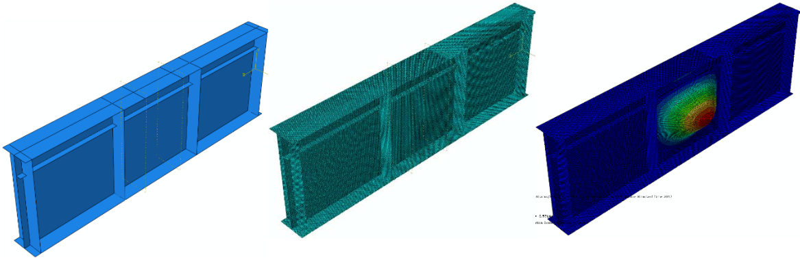
Figure 4. Typical shell-based geometry, mesh and eigenmode-based imperfection.
