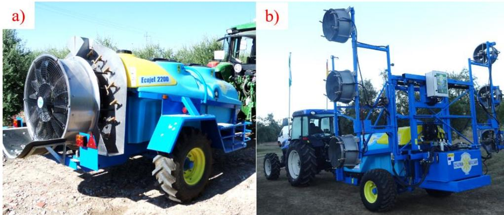
Fig. 3. a. Conventional airblast sprayer. b. Air-assisted sprayer prototype.
