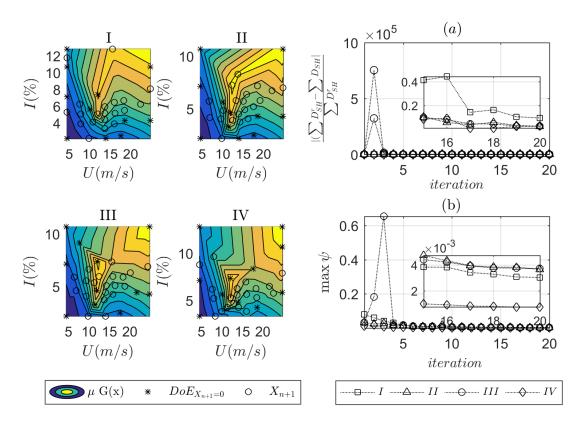
**Figure 8.** Convergence of the Kriging prediction ( $\sum D_{SH}$ ) to the real S-N damage expected in a full year assessment ( $\sum D_{SH}^r$ )
