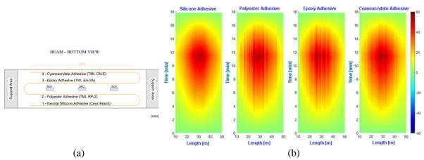
**Figure 5.** Bonded sensors: (a) Setup in the bottom surface of RC beam to be tested statically; (b) Measured strain by different bonded segments of DOFS
