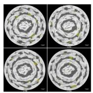
**Figure 2**. μ-CT cross-sectional images along the xy axis of the braided BFRP composite rebar - Void distribution (yellow shaded area) on 4 different z-axis locations
