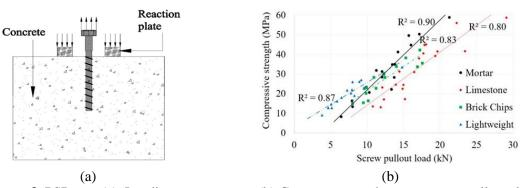
Figure 3. PSP test: (a) Loading arrangement, (b) Concrete strength versus screw pull-out load
