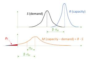
Figure 1. Demand, capacity and failure curves
