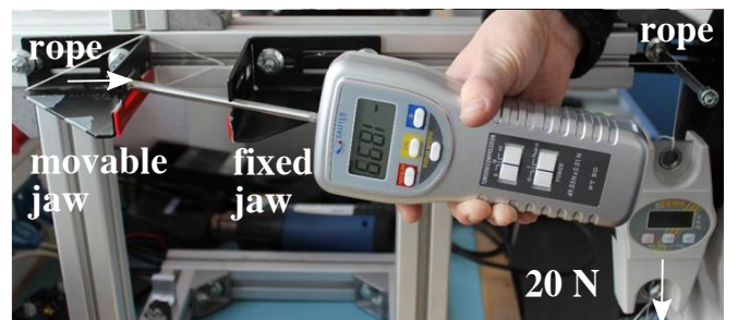
Fig. 8: Test rig to determine the required force for closing the gripper: A weight of 2 kg is converted into a force of 20 N that actuates the left gripping jaw via a rope mechanism
