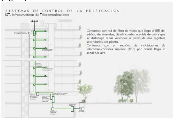
Figure 11: System of Infrastructures for Telecommunication control and automation
