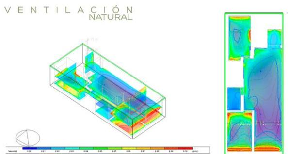
Figure 7: Natural ventilation: indoor air speed (source: Archiwizard Analysis)
