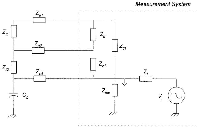
Fig. 4. Equivalent circuit to analyze internal interference coupling.
