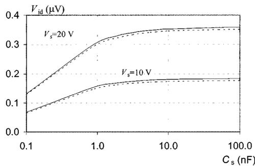
Fig. 6. Differential mode voltage ( $V_{id}$ ) due to internal interference for different values of secondary voltage ( $V_s$ ) and different values of secondary voltage imbalance ( $\Delta V_s = 10\%$  solid line and  $\Delta V_s = 5\%$  dotted line).
