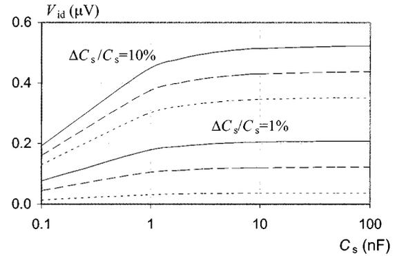
Fig. 5. Differential mode voltage ( $V_{id}$ ) due to internal interference for different values of imbalance of stray capacitance to ground and different values of secondary voltage imbalance when  $V_s = 10$  V ( $\Delta V_s/V_s = 100\%$  solid line,  $\Delta V_s/V_s = 50\%$  dashed line and  $\Delta V_s/V_s = 5\%$  dotted line).
