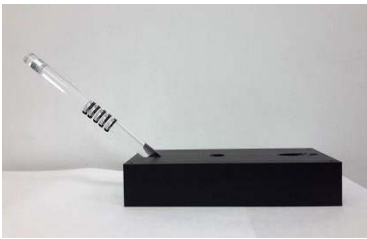
Figure 3: Isotropy test set-up for rings ( \varphi = 40^\circ )
