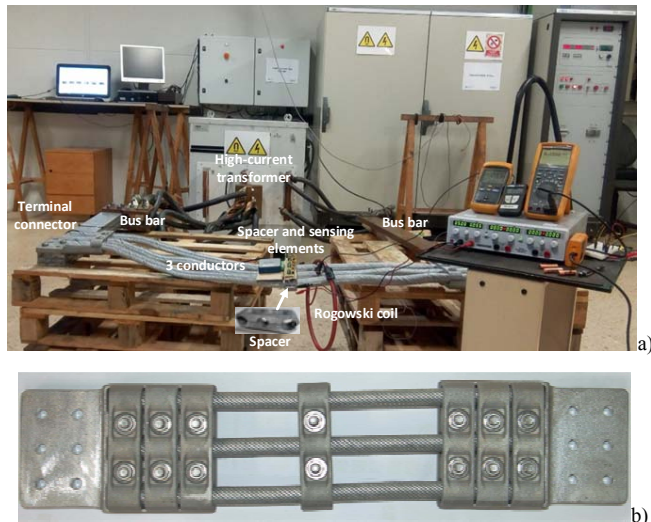
Fig. 7. a) Experimental setup used in this work including the conducting loop with the three conductors, the spacer and the terminal connectors, the high-current transformer and the three Hall sensors. b) Terminal connectors, spacer and the three conductors.
