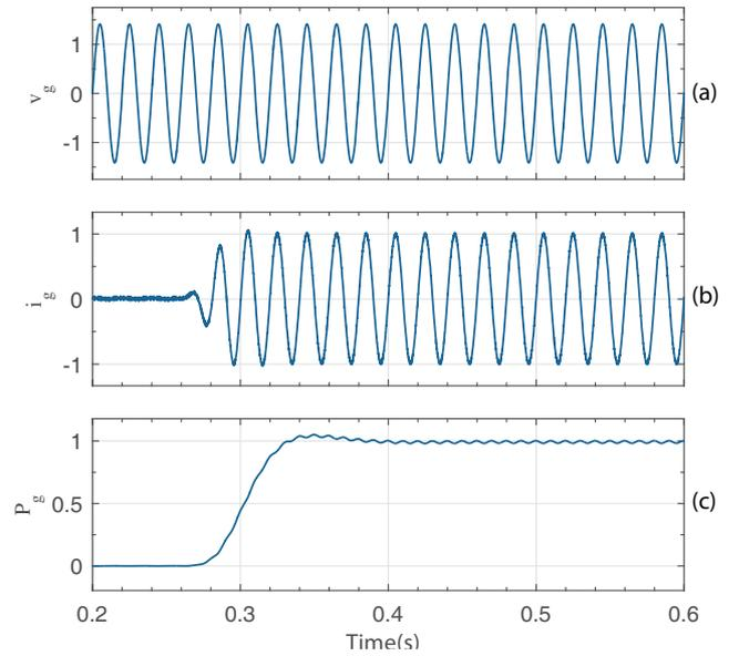
Fig. 8: Grid waveforms. (a) Voltage, (b) Current, (c) Active power
