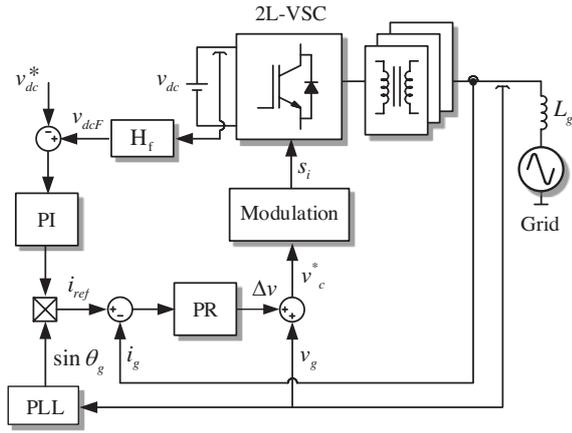
Fig. 5: Single-phase voltage oriented control scheme
