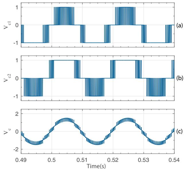
Fig. 6: Voltage waveforms. (a) Converter voltage  $v_{c1}$ , (b) Converter voltage  $v_{c2}$ , (c) Output voltage  $v_c$
