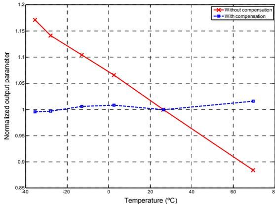
Figure 3. Temperature dependence of the output parameter at  $P = P_{\text{atm}} = 101 \text{ kPa}$ .
