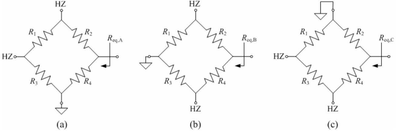
Figure 2. Bridge sensor treated as a resistive circuit and measurement of the equivalent resistances (a)  $R_{eq,A}$ , (b)  $R_{eq,B}$  and (c)  $R_{eq,C}$ .
