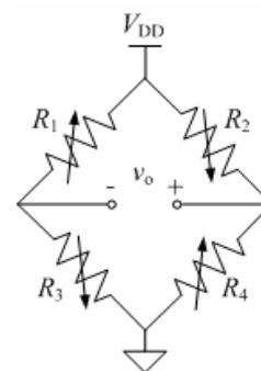
Figure 1. Piezoresistive pressure sensor in a Wheatstone-bridge configuration.
