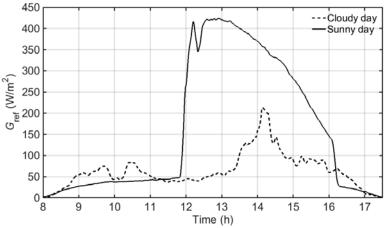
Fig. 14. Irradiance measured by a HD52.3DP147 pyranomenter during a sunny and a cloudy day.
