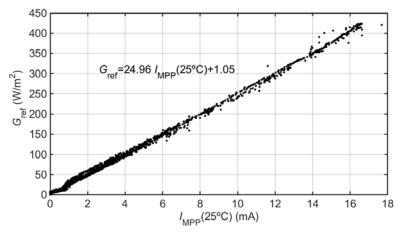
Fig. 16. G<sub>ref</sub> versus I<sub>MPP</sub>(25 °C) obtained during several days and the resulting linear regression.
