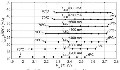
Fig. 7. Temperature compensation of  $I_{\text{MPP}}$ .
