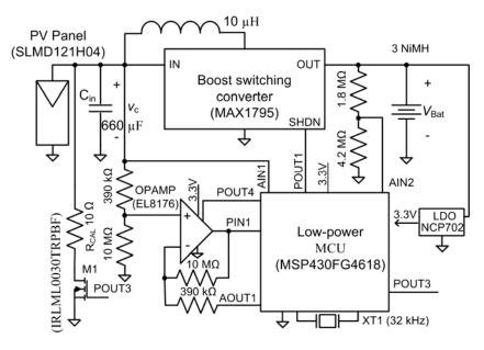
Fig. 8. Circuit diagram of the MPPT system implemented.
