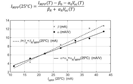
Fig. 6. Dependence of  $\beta$  and  $\alpha$  on  $I_{\text{MPP}}$  (25°C).
