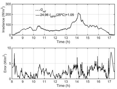
Fig. 17. Comparison between measured and reference irradiance during a cloudy day.
