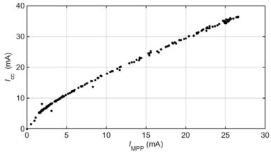
Fig. 4. Measured  $I_{cc}$  versus  $I_{MPP}$  for a SLMD121H04L PV panel at constant temperature (25°C).
