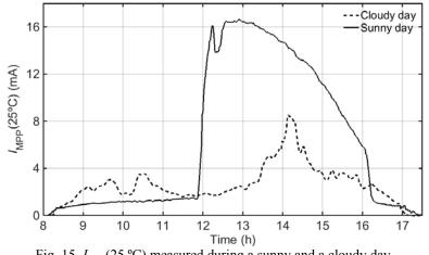
Fig. 15. IMPP(25 °C) measured during a sunny and a cloudy day.
