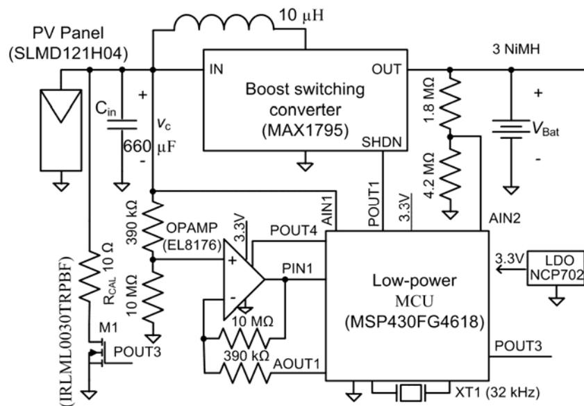
Fig. 8. Circuit diagram of the MPPT system implemented.
