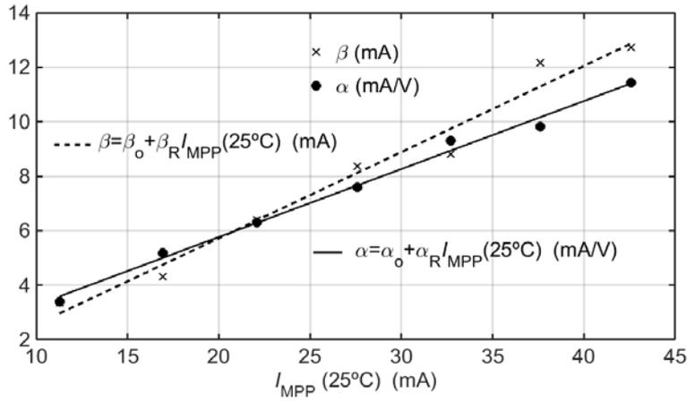
Fig. 6. Dependence of  $\beta$  and  $\alpha$  on  $I_{MPP}(25^\circ\text{C})$ .
