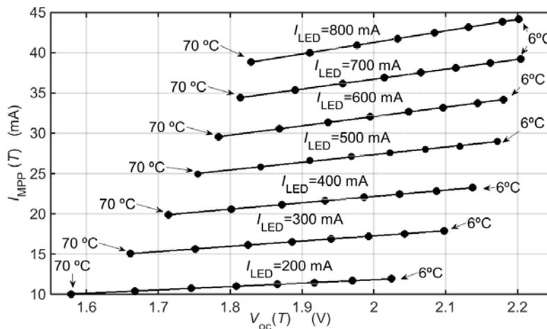
Fig. 5. Temperature dependence of  $I_{MPP}$  for SLMD121H04.
