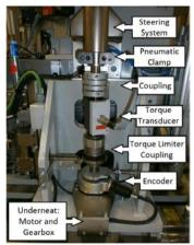
Fig. 1. EOL test machine that performs the friction test for steering systems.
