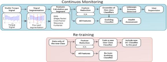
Fig. 5. Proposed methodology for the EOL test machine. The monitoring method is composed by a signal processing stage where statistical features are calculated and analyzed by a novelty detection and a multi-fault classification models to assess the condition of the machine.
