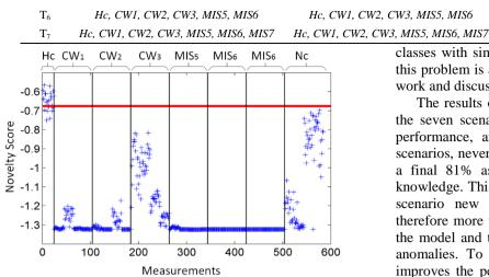
Fig. 6. Resulting Novelty Score of the T1. The red line is the novelty threshold, Th, which is set to -0.67. The black lines represent the division among the different classes during the test.
