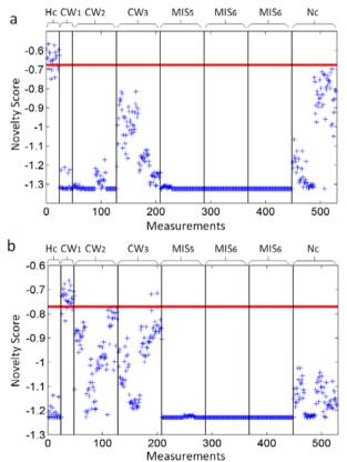
Fig. 7. Resulting Novelty Score of the  $T_2$ . The red line is the novelty threshold, *Th*, which is set to -0.67 for the first OC-SVM and -0.77 for second. The black lines represent the division among the different classes during the test. a) The novelty results of the OC-SVM trained using measurements of the *Hc* class. b) The novelty results of the OC-SVM trained using measurements of the *CW<sub>I</sub>* class.
