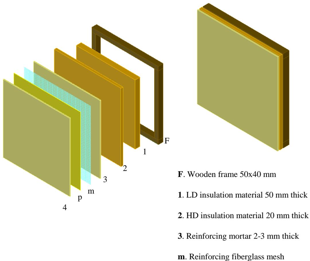
*Figure 1. Schema of the ETICS incorporating bio-based insulations prepared for the tests. In the case of the EPS, layers 1 and 2 had the same density (LD).*
