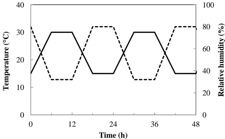
Figure 5. Schema of the run performed. Solid line corresponds to temperature and dotted line to relative humidity
