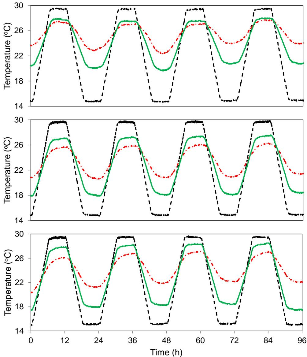
Figure 10. Temperatures  $T_{se}$  (black dashed line),  $T_{int}$  (green solid line) and  $T_{si}$  (red dot-dashed line) for the three ETIC systems; corn pith (top), wood (middle) and polystyrene (bottom) for 4 cycles (temperature shift from 15 to 30°C and RH from 80% to 32%).
