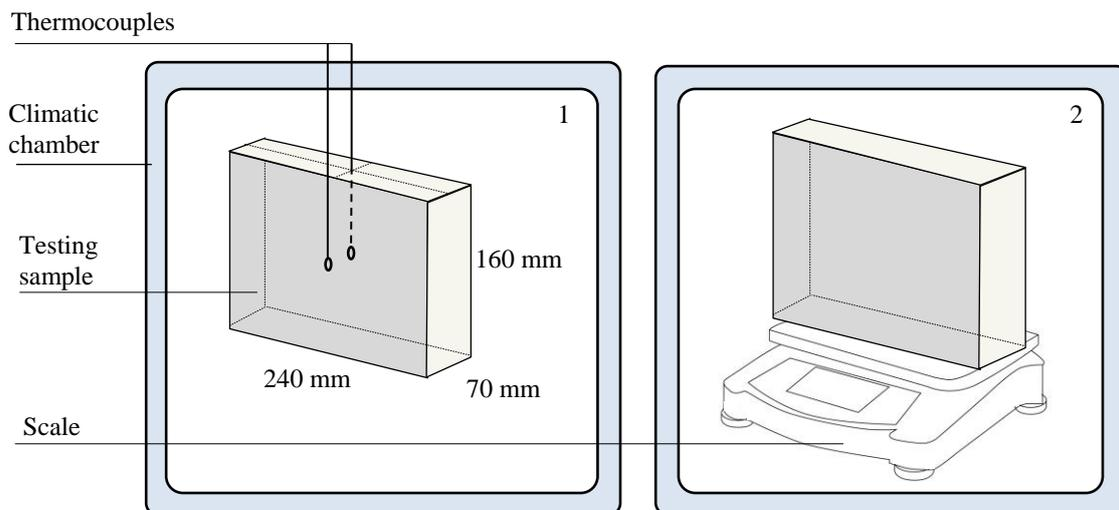
Figure 2. Schema of the experimental set up.
