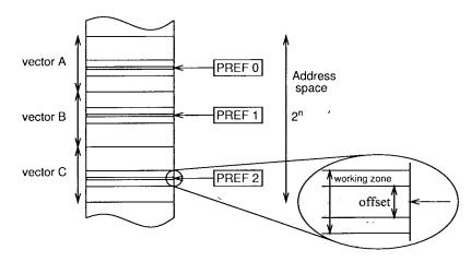
Fig. 1. Address space with three vectors.
