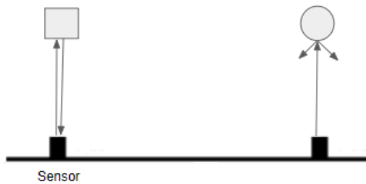
Figure 32: Echo behaviour depending on the shape.
