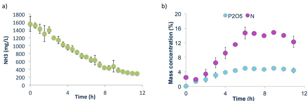
Figure 2. a) Ammonia evolution in the feed side and b) N and P<sub>2</sub>O<sub>5</sub> evolution in the stripping side over time.
