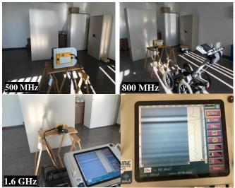
Fig. 2. GPR data acquisition for the zero-time position test using three antennas (500 MHz, 800 MHz and 1.6 GHz).
