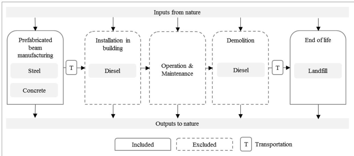
Figure 2. Diagram of the system boundaries for the environmental analysis of beams.
