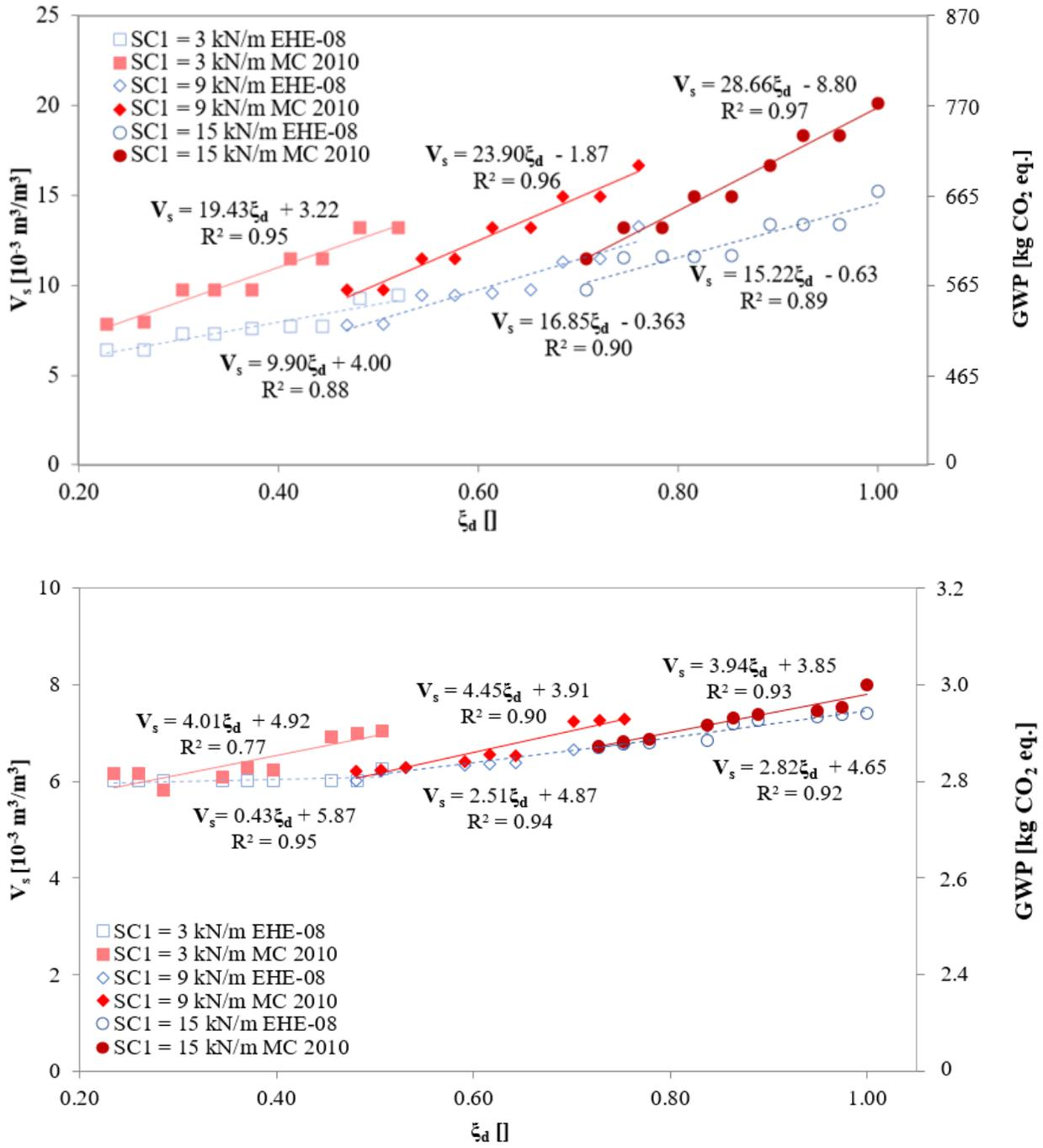
Figure 3.  $V_s - \xi_d$  relationships for: (a, top)  $L = 8.0 \text{ m}$ ,  $h = 0.6 \text{ m}$  and  $f_{ck} = 35 \text{ N/mm}^2$  and (b, bottom)  $L = 12.0 \text{ m}$ ,  $h = 1.0 \text{ m}$  and  $f_{ck} = 50 \text{ N/mm}^2$ .
