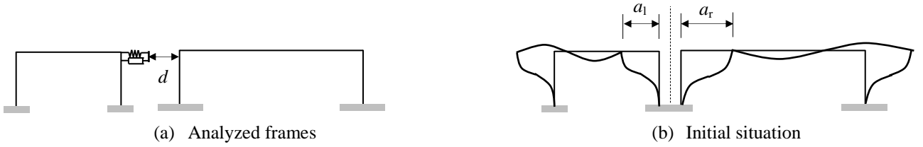
Figure 4. Colliding frames considered in the comparison parametric study
