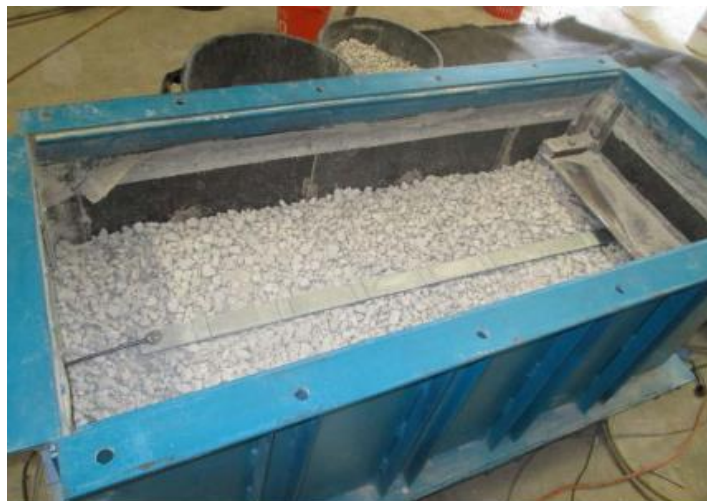
Figura 1.5.2 Reforç i caixó utilitzats. (Font: Pullout Resistance of Mechanically Stabilized Earth Wall Steel Strip Reinforcement in Uniform Aggregate )
