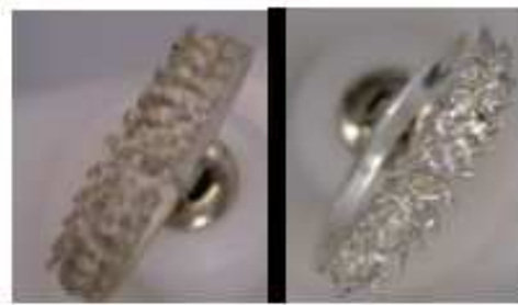
Figure 95. Silver ring before/after being polished with the electro-mechanical polishing machine. Source: Own
