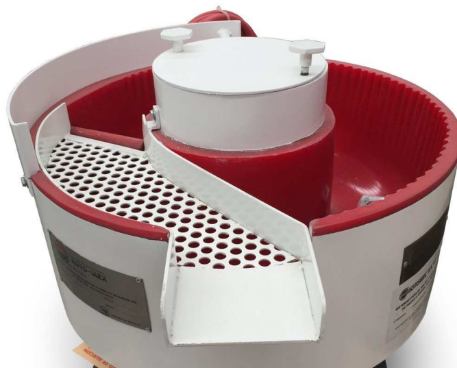
Figure 59. Vibratory machine with the system flow-through, which automatically separates media and pieces.
