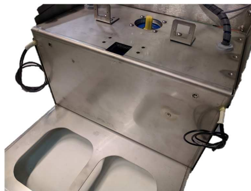
Figure 83. Electrical cabinet plate separator. Source: Own
