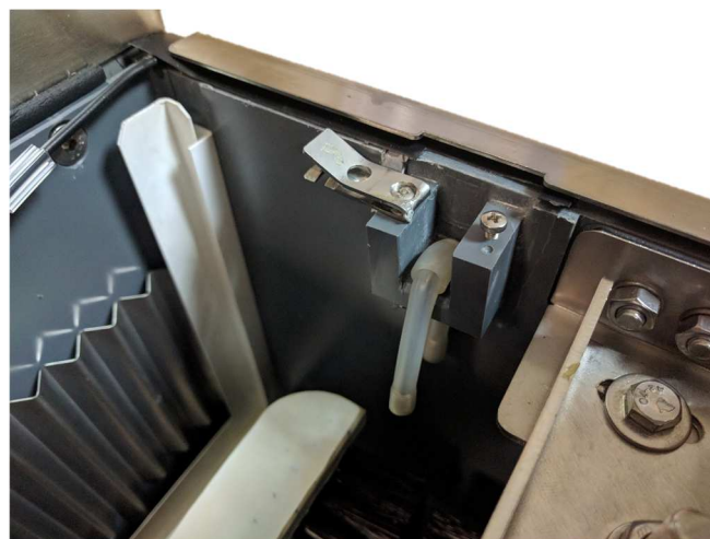
Figure 87. Anodic connection to the rack, fitted inside the working tank. Source: Own
