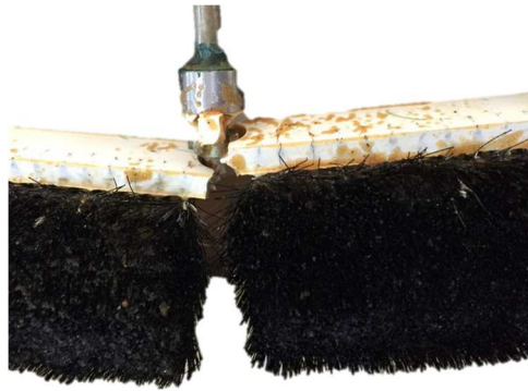
Figure 112. Broken sliding brush due to fatigue. Source: Own
