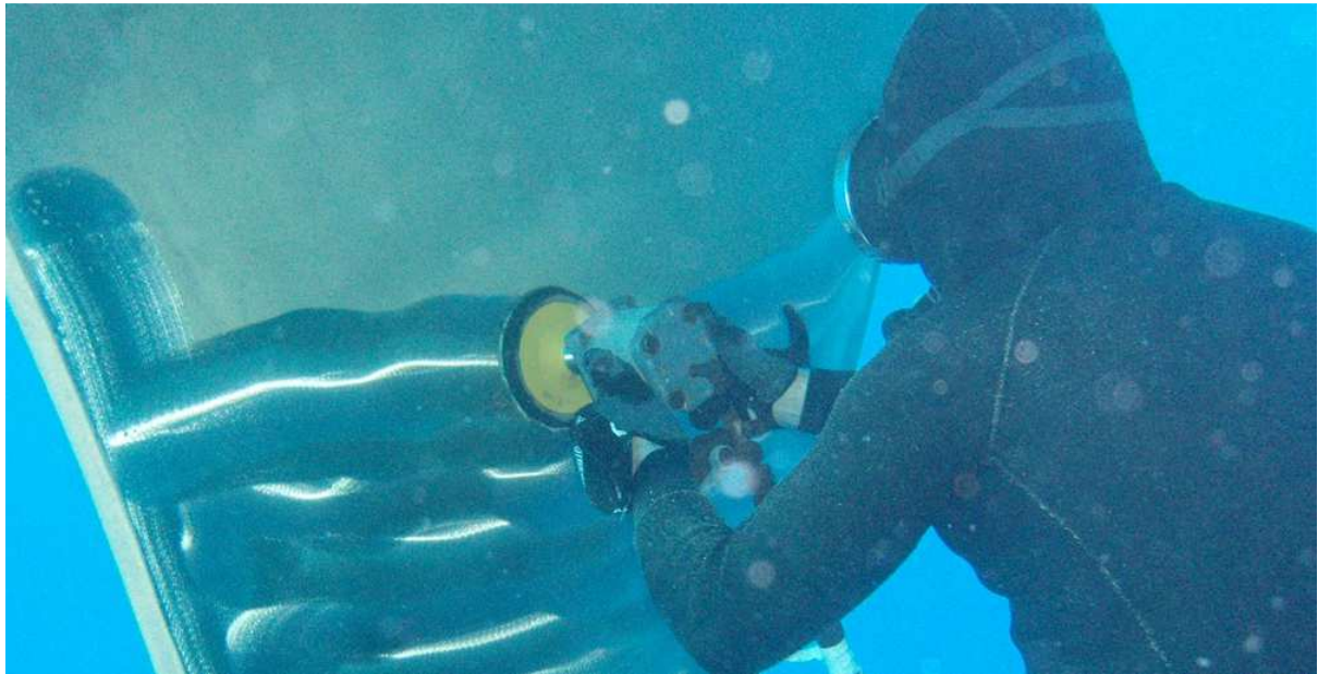
Figure 40. Polishing a bronze propeller inside the water with an angular grinding machine. Source: www.dynamicdivers.gr
