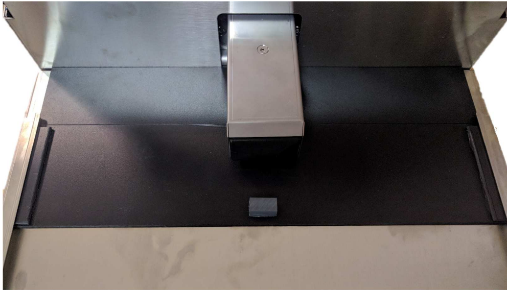
Figure 103. All the protections against the splashing fitted in the machine. Source: Own
