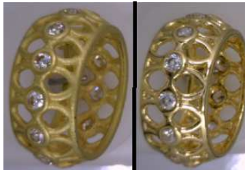
Figure 76. Gold ring before/after being polished with the electro-mechanical polishing machine. Source: Own
