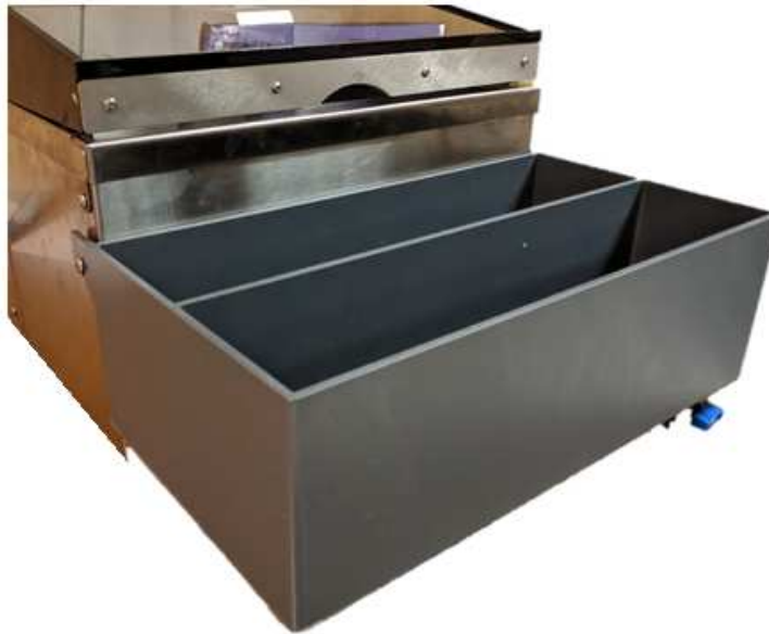
Figure 93. Rinsing tank fitted in front of the EN-34. Source: Own
