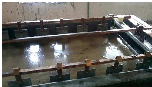
Figure 74. Electro-polishing tank with cathodes placed inside the bath. Source: www.indiamart.com
