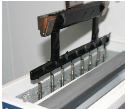
Figure 75. Anodic rack inside the tank. Source: www.techinc.com
