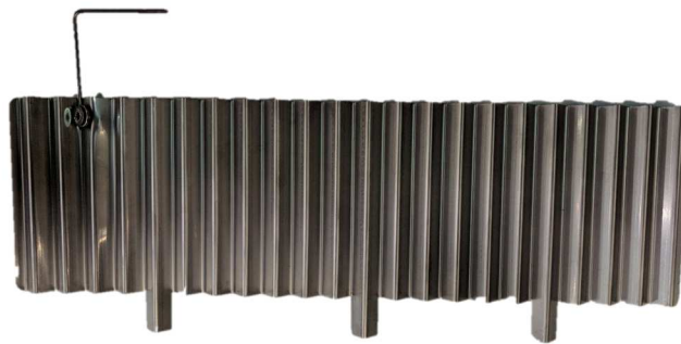
Figure 88. Stainless steel cathode. Source: Own
