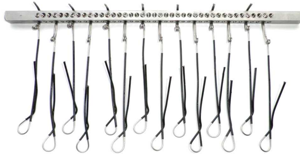
Figure 79. Anodic rack with hooks, where the pieces are hanged. Source: Own
