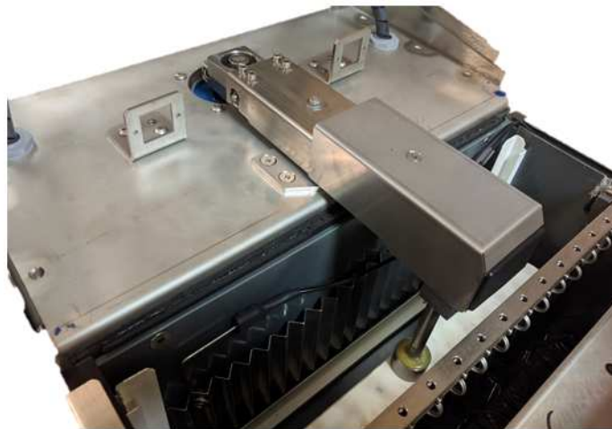
Figure 92. Driving head fitted on the electrical cabinet plate separator, with the brush at its end. Source: Own
