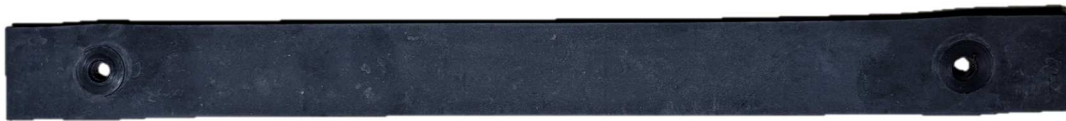
Figure 106. Junction used between the working tank and the electrical cabinet plate separator, which prevents wall bending. Source: Own
