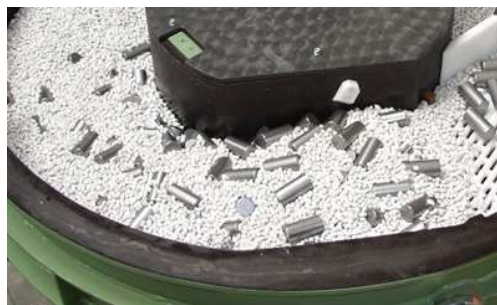
Figure 57. Mix of pieces and media inside a vibratory machine. Source: www.interempresas.net
