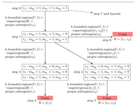
**Fig. 9** Several steps of the execution of Algorithm 5 on the TS U of Fig. 8(b) with k=1. Each step shows the contents of the stack s if the SMT problem was feasible, otherwise it shows the set of minimal regions found so far. The label on each arc indicates which SMT problem is solved in each case.
