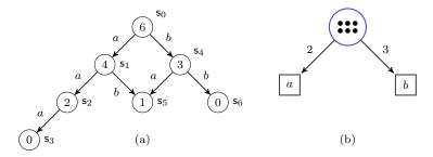
Fig. 7 (a) Transition system for the log  $\{aaa, ab, ba, bb\}$  and one of its regions r:  $r(s_0) = 6, r(s_1) = 4, \ldots, r(s_6) = 0$  in which the gradients of the events are  $\delta_r(a) = -2$  and  $\delta_r(b) = -3$ . (b) Corresponding feasible place in the Petri net.
