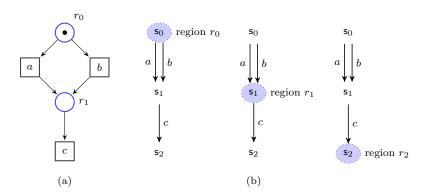
**Fig. 8** (a) A PN. (b) Its reachability graph (three copies), in which three regions, that form the set of minimal regions, have been shaded (e.g., region  $r_0$  is  $r_0(s_0) = 1, r_0(s_1) = 0, r_0(s_2) = 0$ ).
