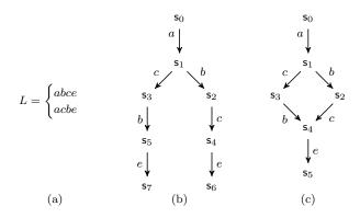
Fig. 6 (a) A log. (b) Transformation of the log into a transition system, merging equal prefixes of sequences. (c) Transformation of the log into a transition system, merging prefixes with the same number of the same activities.
