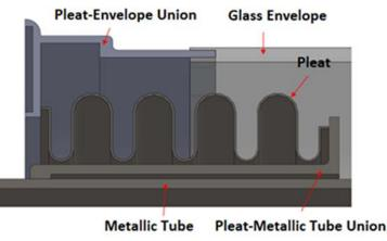
Figure 2: Inner design of the heat collecting elements in the simulation.
