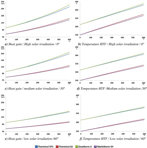
Figure 4: Oils' heat gain and temperature increase through the PTS
