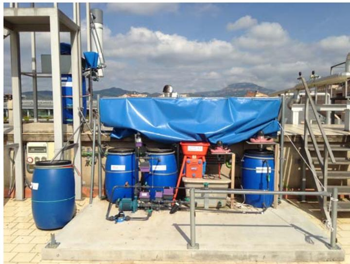
*Figure 1: Prototype of the water purification plant.*
