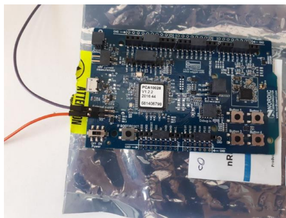
Fig. 3.18. Supply Voltage and ground wires connected from the power analyser to the DK External Supply pins (1)
