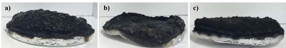
**Figure 11:** Photographs of the ABS flame retardant formulations residue after the cone calorimeter test.
