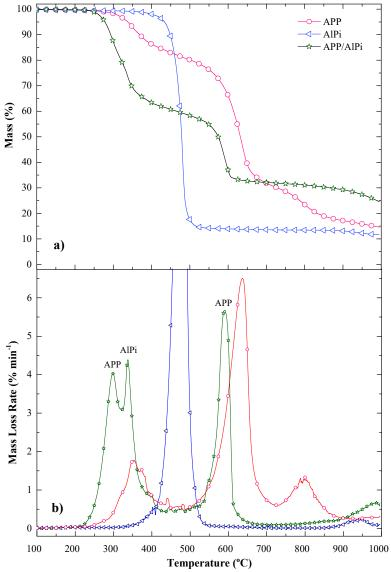
Figure 1: TG a) and dTG b) curves of APP, AlPi and APP/AlPi obtained at 10°C/min under N<sub>2</sub>.
