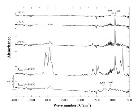
Figure 6: FT-IR spectra of ABS-APP pyrolysis products at the temperature of the maximum mass loss rate and at the beginning of decomposition.
