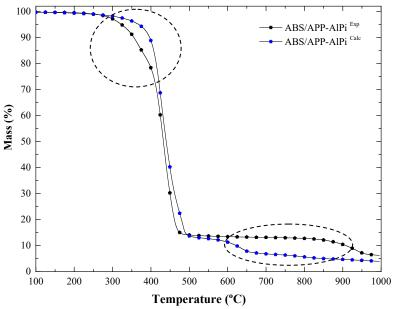
Figure 3: Experimental and calculated TG curves of ABS-APP/AlPi system.
