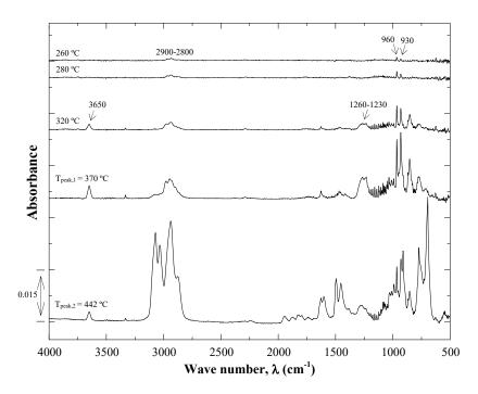
Figure 8: FT-IR spectra of ABS-APP/AlPi pyrolysis products at the temperature of the maximum mass loss rate and at the beginning of decomposition.
