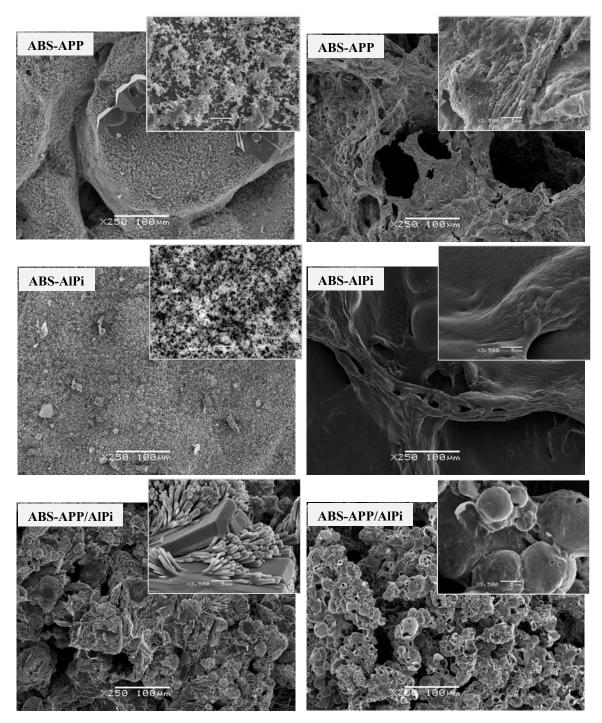
Figure 12: SEM micrographs of the upper (left) and down surface (right) of the ABS phosphorus flame retardant samples after the cone calorimeter tests (at  $250 \times$  and  $3500 \times$ , with a scale bar of 100 and 5  $\mu$ m respectively).
