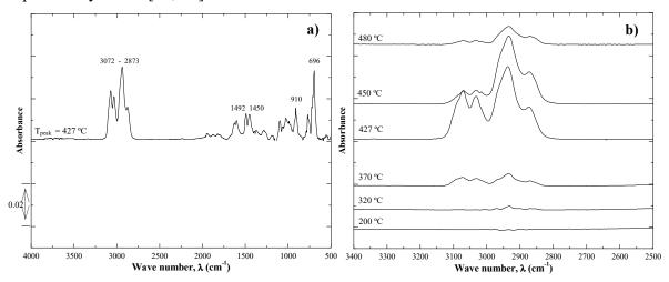
Figure 5: FTIR spectra of ABS pyrolysis gases obtained at a) the temperature of maximum mass loss rate and at b) different temperature between 3400 cm<sup>-1</sup> and 2500 cm<sup>-1</sup> of wavenumber.
