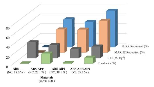
Figure 10: Comparative of the main flammability and fire behavior results of each material, obtained from UL-94, LOI and cone calorimeter tests.
