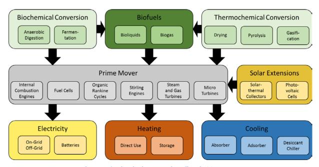
Figure 1 Key components in biomass-fired and solar assisted small-scale CCHP systems
