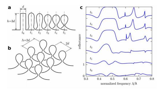
Fig. 3. (a) Time evolution (numerical calculations) of a silicon cylinder during annealing. The time snapshots do not correspond to equal time increments. The time  $t_0$  corresponds to the initial cylinder before annealing. (b) Schematic of the studied metasurface; a square array,  $\Lambda$ =2*d*, of pedestalled spheroids. (c) Calculated reflectance at normal incidence of a metasurface considering the different pedestalled shapes in panel (a).
