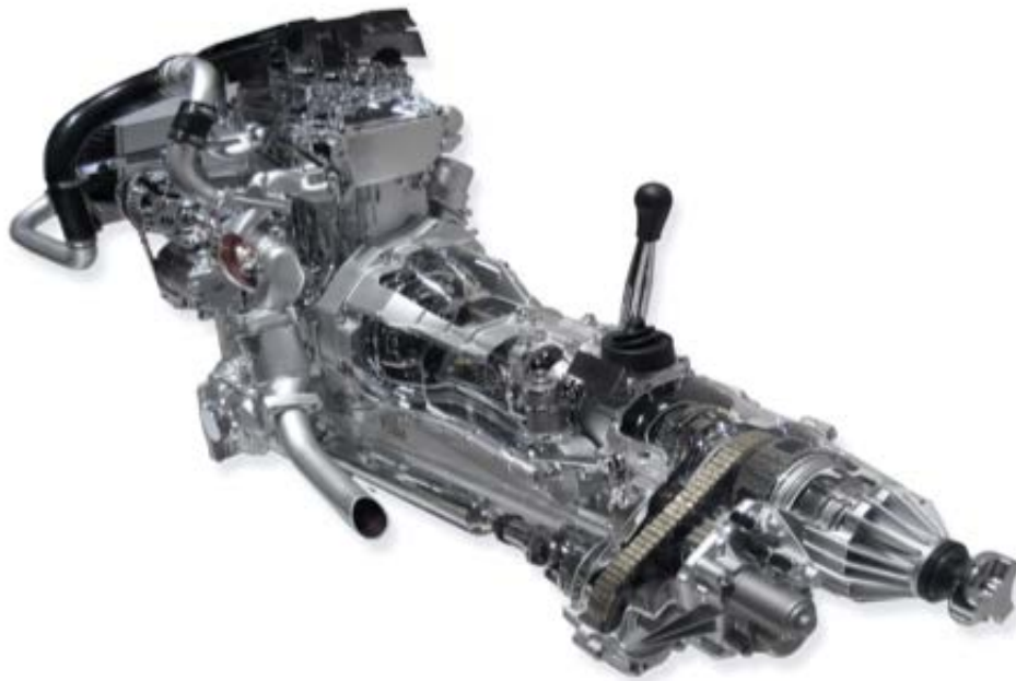
Figure 1. Nissan Pathfinder Engine. Characteristics: (i) 747 parts and 330 references (ii) 378 elemental assembly tasks grouped into 140 production line tasks.
