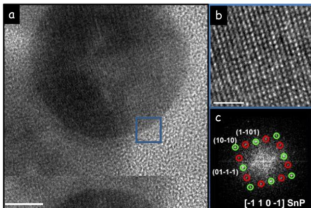
Figure 2 a) HRTEM micrograph of a SnP NC with the trigonal structure; b) Detail of the NC area squared in blue; and c) its corresponding power spectrum. In the power spectrum, besides the indexed spots (circled in green), some extra spots (circled in red), which should not exist in the pure hexagonal structure, were found.
