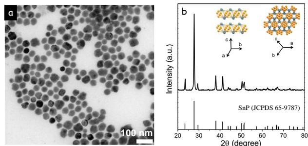
Figure 1. TEM micrograph (a) and XRD pattern (b) of the NCs produced from the reaction of tin oxalate with HMPT at 270 °C and in the presence of TDPA: TDPA/Sn = 1. Inset within the XRD graph shows the SnP crystal structure along two different directions.
