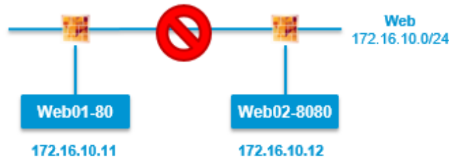
Figure 126. Isolating two VMs remaining to a single network using a firewall rule.
