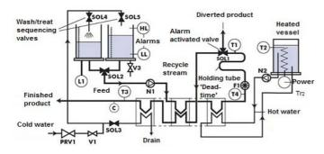
Fig. 2. Process flow diagram for the pasteurizing process [2].
