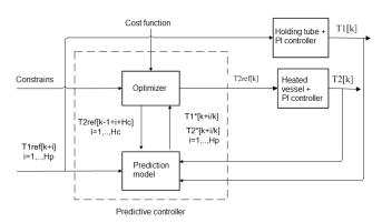
Fig. 4. Model Predictive Control as Supervisor Topology.
