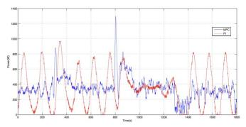
Fig. 9. Heater power consumption for both control topologies. Total energy consumption was computed as the area under the curve.
