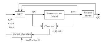
Fig. 6. Representative block diagram of single-layer MPC with fatigue model and linear regulator.
