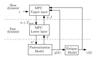
Fig. 7. Representative block diagram of two-layer MPC with fatigue model.
