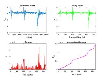
Fig. 3. Rainflow counting damage estimation.
