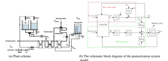
Fig. 1. Plant scheme and control block diagram of the pasteurization plant.
