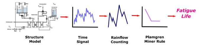
Fig. 2. Rainflow counting damage procedure.
