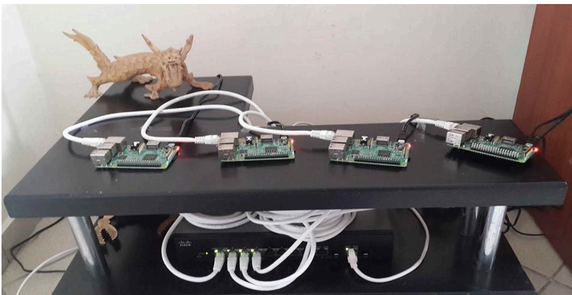
Figure 5. HPRC hardware platform. HPRC cluster with four Raspberry PI 3 model B deployed using the HPC-ROS package.
