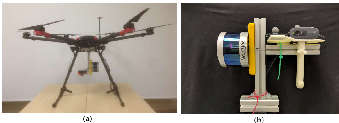
404 Figure 11. Hardware Prototypes: (a) Early prototype UAV hexacopter deploying the sensor setup 405 considered in this work; (b) hand-held sensor rigid body for experimentation in flight-denied areas 406 (indoor laboratories, etc...).
