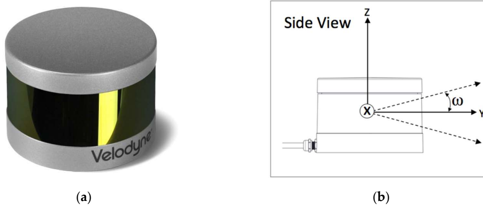
154 Figure 3. Sensor Velodyne VLP16: (a) appearance of the sensor; (b) sensor coordinate frame, with 155 origin and scan width detail.
