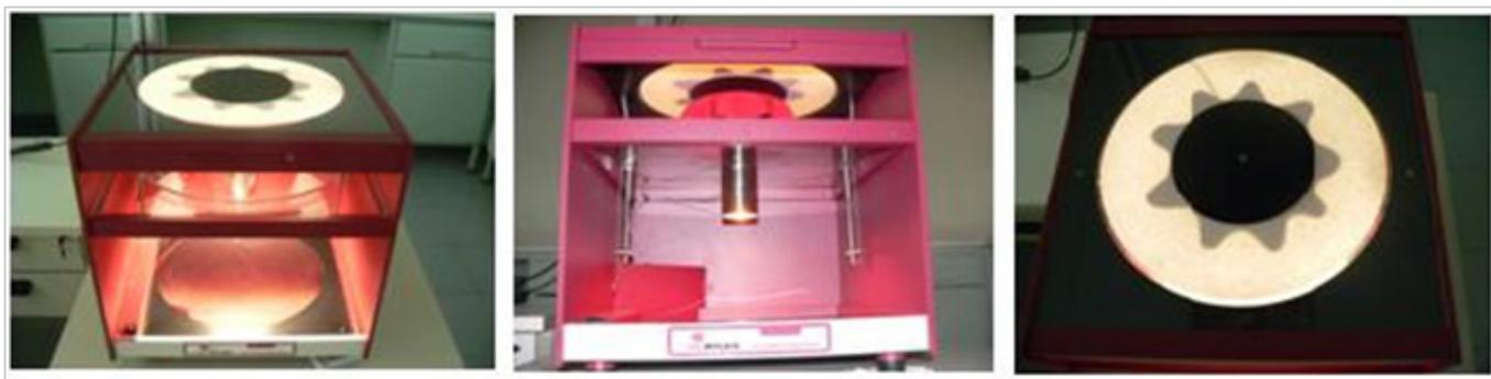
Figure 1. Current design of the Cusick drape meter (Photo: Department of Textile and Paper Engineering, UPC)
