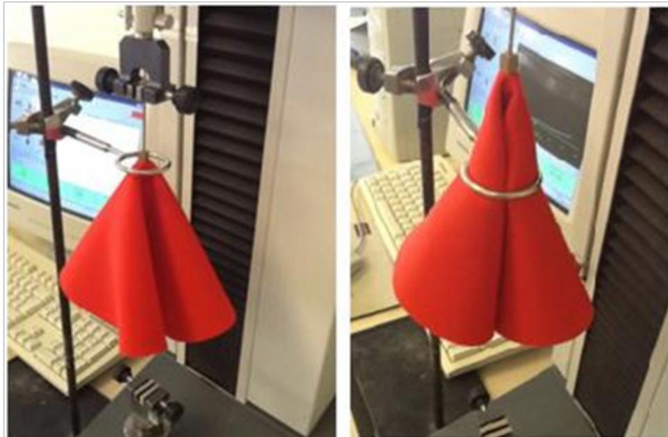
Figure 5. Sequence of the UPC ring method. (Left) Start of the test. (Right) During the test
