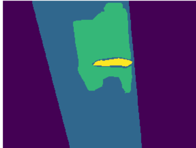
Figure 12: Label of sample of data based on the intersection of each original label. Green represents the intersection area of delamination, yellow the rebar exposure intersection, blue non damage intersection and purple represents the don't care area.
