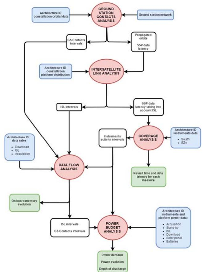
FIGURE 4. Detailed performance analysis and simulation flow diagram for each configuration (defined by its identification number -ID-).
