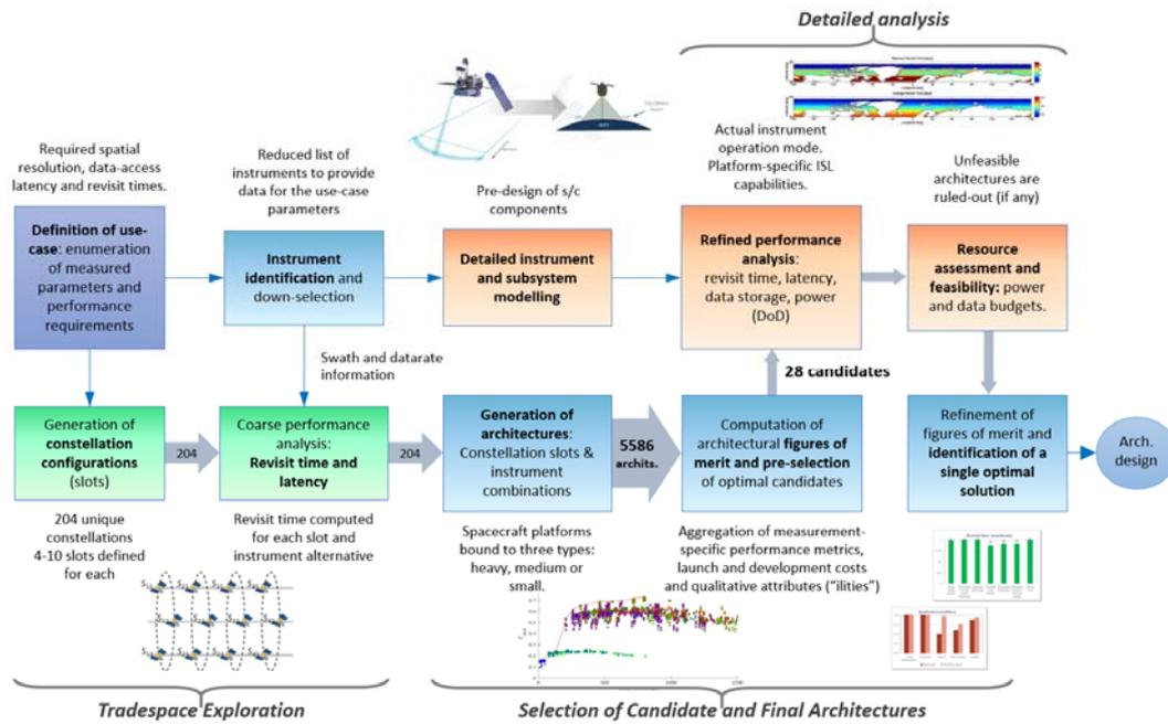
FIGURE 2. Graphical explanation of the Systems Architecture Study to select the optimum configuration.
