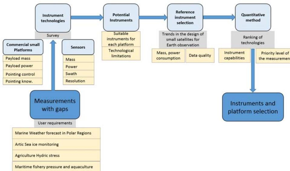
FIGURE 3. Instrument and platform selection process to meet the user observation requirements.
