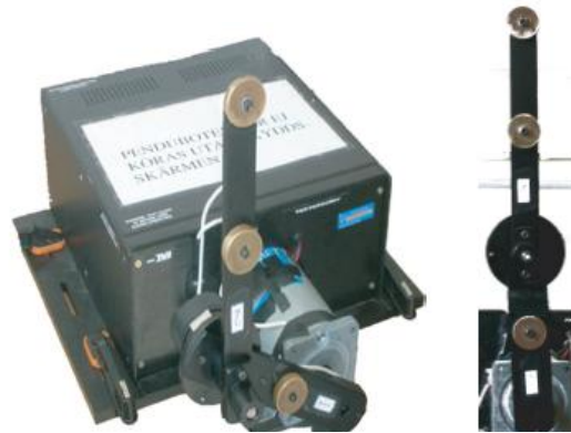
Fig. 4.2. Pendubot connected to the motor (left), Pendubot fully extended (right) [7].
