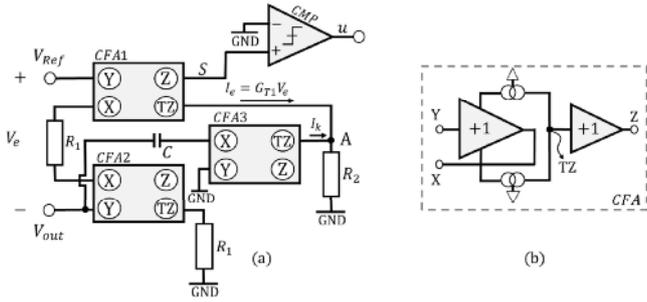
Fig. 5. (a) Proposed analog implementation of SM controller block based on CFA, (b) equivalent block for the CFA.
