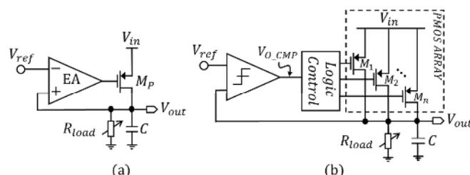
Fig. 1. Block diagram of different types of LDOs, (a) analog LDO (b) digital LDO.
