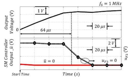
Fig. 9. Start-up response of the proposed regulator based on the SM controller.
