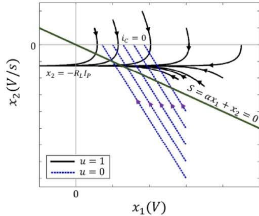
Fig. 4. Phase plane of the substructure corresponding to both  $u=1$  and  $u=0$  for different starting positions  $(x_1, x_2)$ .
