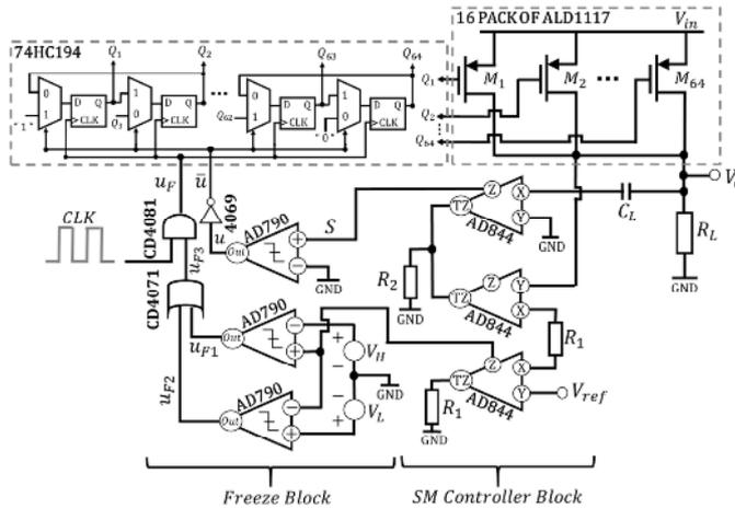
Fig. 6. The complete schematic diagram of the proposed regulator based on the sliding-mode controller.
