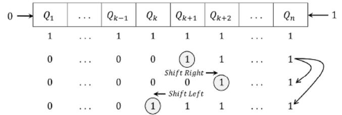
Fig. 3. Operation of the bi-directional shift register.
