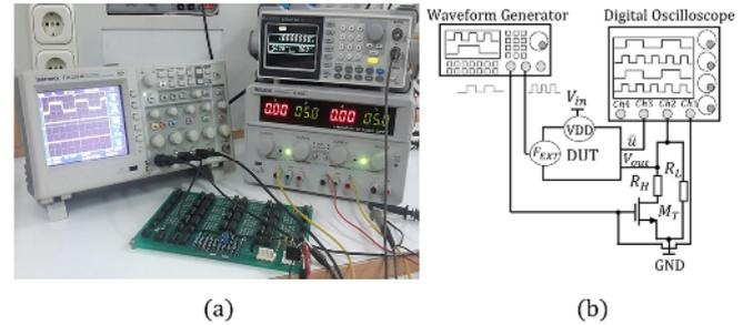
Fig. 8. (a) Lab measurement components, and (b) measurement setup.
