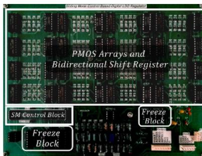
Fig. 7. The implemented PCB of the proposed regulator based on the SM controller.
