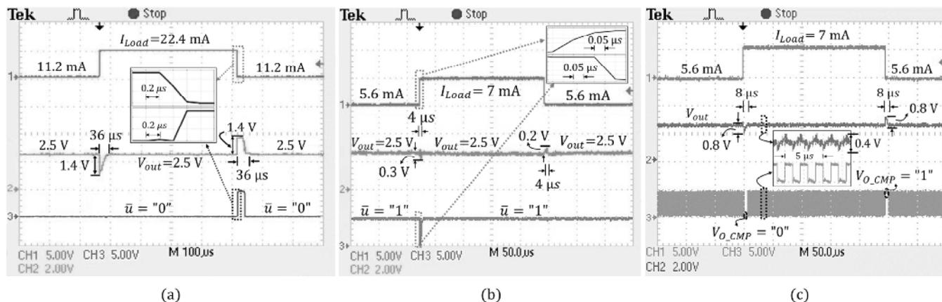
Fig. 10. Transient response of the proposed regulator based on the SM controller at 1 MHz clock frequency when the current changes from (a) 11.2 mA to 22.4 mA, (b) 5.6 mA to 7 mA, and (c) transient response of the regulator based on the conventional linear control (Fig.2 (b)).
