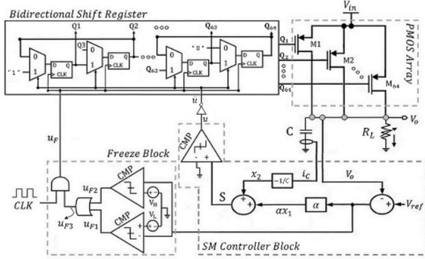
Fig. 2. Proposed QDLDO regulator based on the SM controller.
